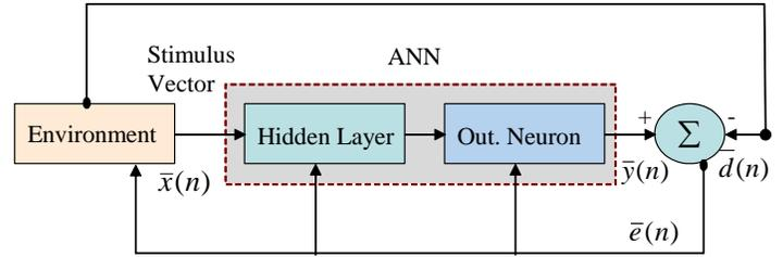
Figure 2. Generalized ANN block diagram simulating two diverse learning paradigms adapted from [19].
