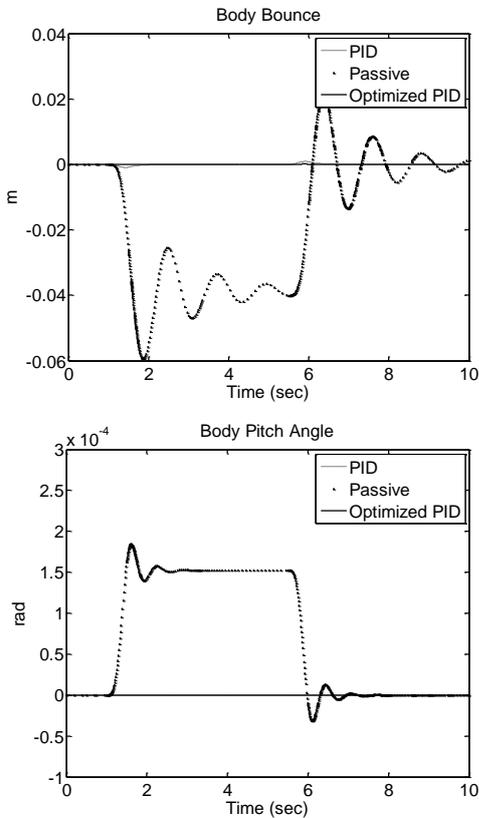
Figure 6. Half-car response due to inertial forces generated with car cornering situation- PID control schemes.
