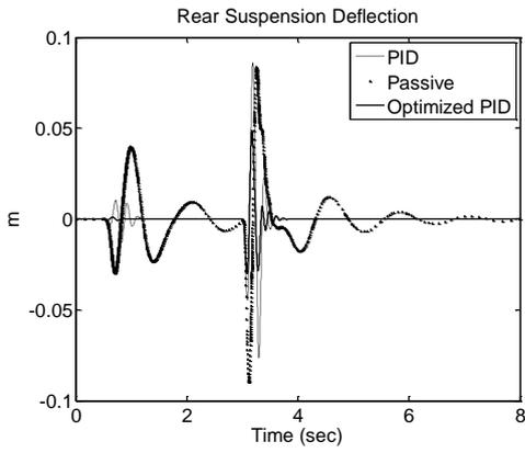
Figure 5. Half-car response of PID control schemes for an 11 cm bump.
