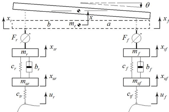
Figure 2. Proposed half-car active suspension system.
