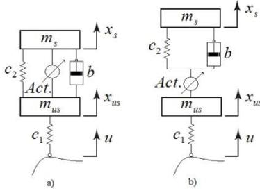
Figure 1. Active suspensions: a) high bandwidth (parallel), b) low bandwidth (series).
