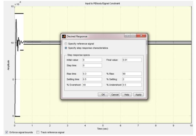
Figure 4. Desired step response for optimized PID control.
