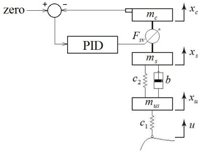
Figure 3. PID control scheme for car body.
