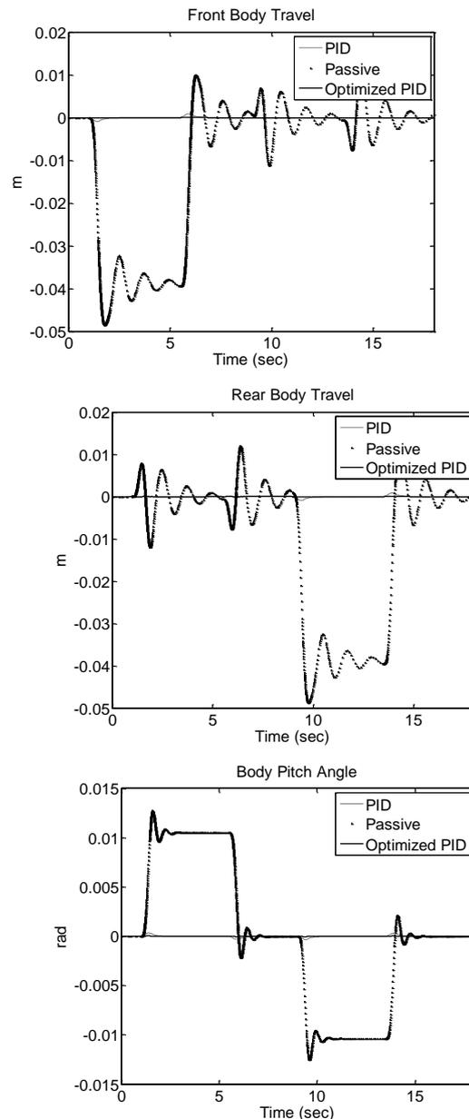
Figure 7. Half-car response due to inertial forces generated in car body braking (t=[1,6]sec) and acceleration (t=[9,14]sec) situations.
