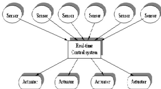
Figure 1: General model of a real-time system [1].
