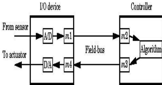
Figure 2: Schematic drawing of a communication delay [2].
